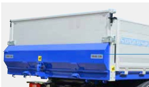
Top-hung spreader gate with automated steel tailgate
