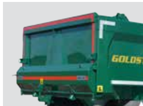
Top-hung, pivoted or high opening spreader gate
